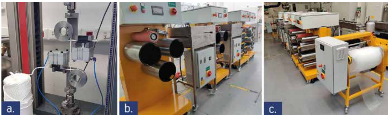
Figure 3: The designed and manufactured twine tensile testing grip during a twine test (left) and the laboratory stretching line (centre and right)
