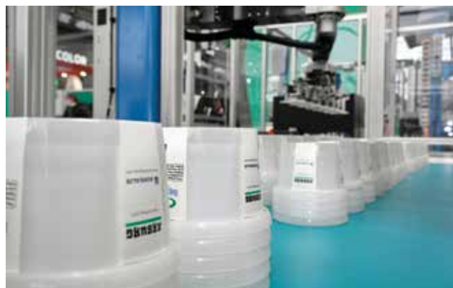
A hybrid Allrounder 1020 H in the packaging version produces IML cups that can be sorted using digital watermarks (“HolyGrail”).
